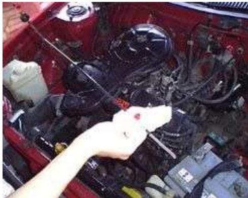
Wipe it off with a clean lint free rag. Then insert it back carefully all the way down into its place.
