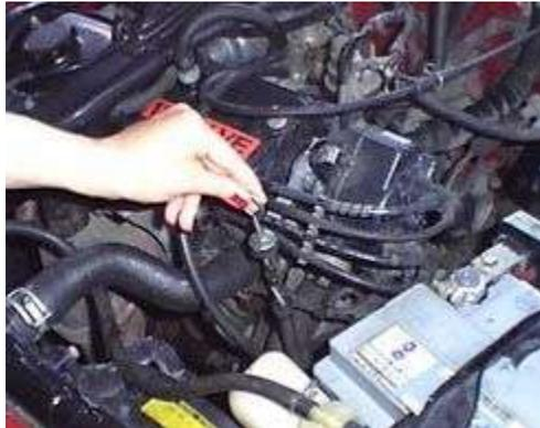
Place your car at a level surface and engage the parking brake. Start the engine. Set transmission shifter in "P" (Park) position, and let the engine idle (on some cars this procedure may be different, check the owners' manual for details). Pull the transmission dipstick. Check your owner's manual to find where transmission dipstick is located in your car.
