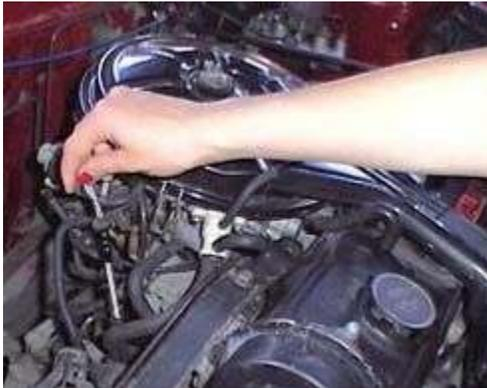
Place your car at the level spot. Stop the engine. Wait for a while to let the engine oil to pour down to the oil pan. Pull the engine oil dipstick. If you don't know where your engine oil dip-stick is, check your owner's manual, usually it has a bright handle saying "engine oil".
